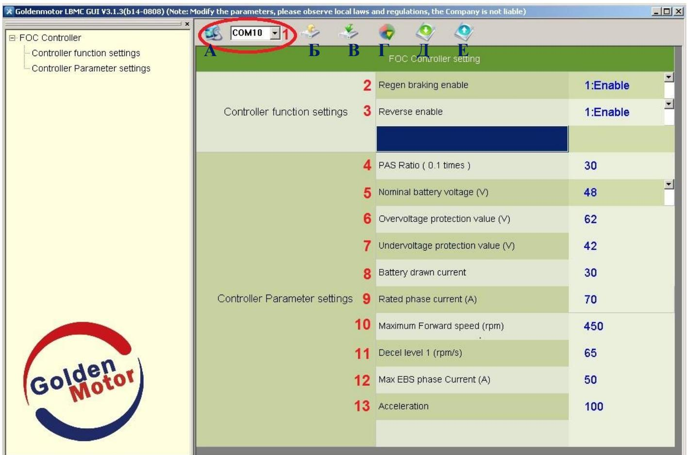
Goldenmotor LBMC GUI V3.1.3(b14-0808) (Note: Modify the parameters, please observe local laws and regulations, the Company is not liable)
